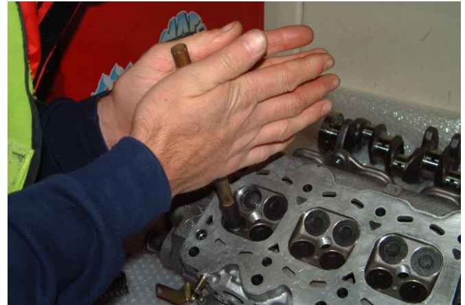
Lapping in the valves using a rubber sucker
