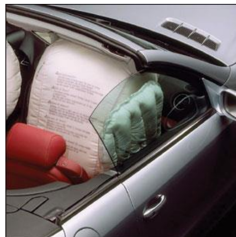
Dual stage passenger airbag. With a warning about undeployed second charges printed on the airbaa itself.
