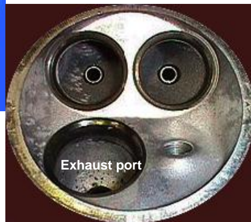
Nissan three valve combustion chamber, one exhaust port and two inlet ports
